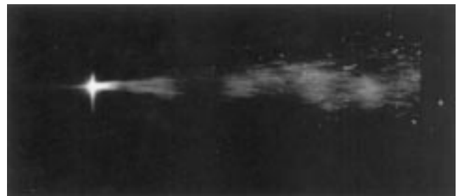
Fig. 8 Photograph taken with a 35 mm film of the particle jet in the wire arc process
